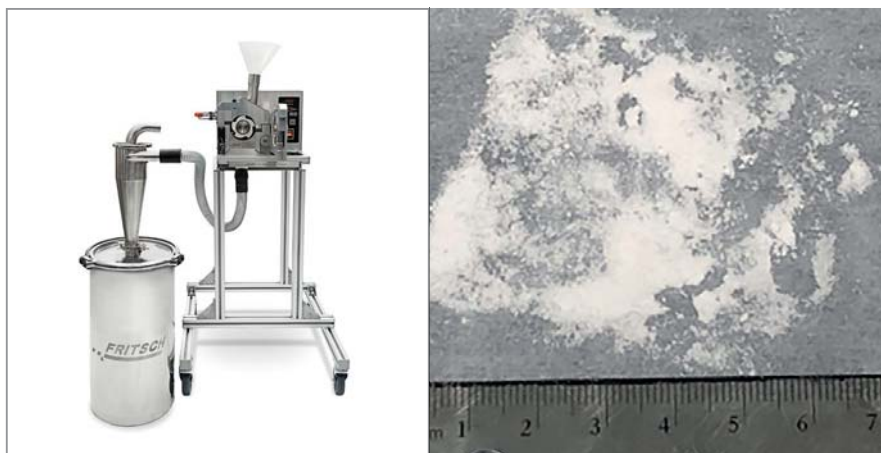
Figure 2. Left – PULVERISETTE 19 cutting mill system, shown with high performance Cyclone collector mounted to 60 L collection tank. Right – CBD isolate homogenized into the low-mid micron range using the P19 system.
