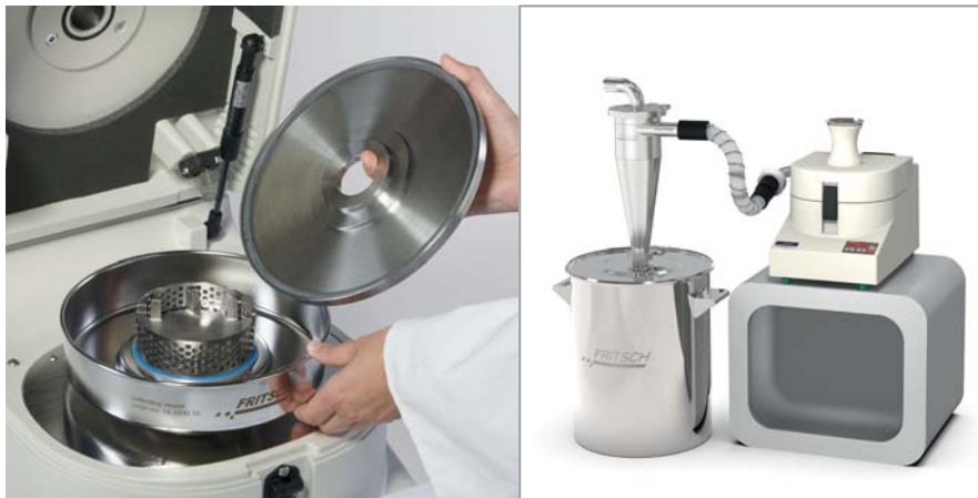
Figure 1. Inside of a PULVERISETTE 14 rotor mill, showing fixed collection pan, rotor, and sieve ring. High performance Cyclone sample collector in stainless steel is shown on the right. Used together with modified collection pan, the P14 system and Cyclone allow continuous feeding and homogenization of CBD material into the low micron range (consistency of talcum powder).
